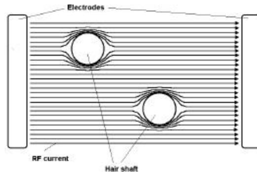
**Figure 3. Current density distribution around the hair shaft.**
